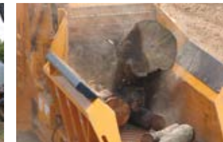
WIDE INFEEED PULLS IN LARGE-DIAMETER MATERIAL
