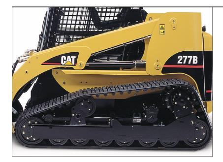
**Rubber Track Undercarriage.** The rubber track undercarriage transfers machine weight to the ground through 48 wheeled contact points on the 277B and 42 on the 287B. Machine weight is evenly distributed throughout the track.
