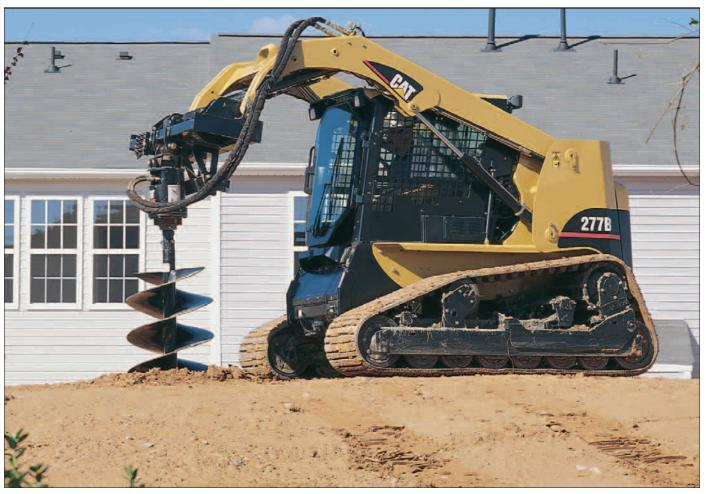
**Front Hydraulics.** Standard ON/OFF front hydraulics are featured on both the 277B and 287B. Optional proportional front auxiliary hydraulics are also available on these models.
