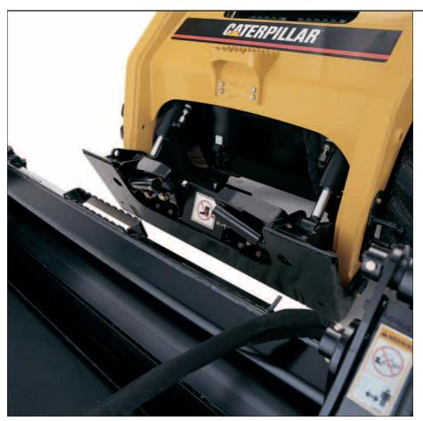
**Quick Coupler.** Work tools can be changed quickly and easily with the Cat Multi Terrain's quick coupler system. The universal coupler interface features:
