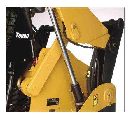
**Lift Arms.** The loader lift arms are purposedesigned to provide a substantially straight load path into the machine and a good viewing area to the work tool and sides of the machine. The lift arms are also designed to handle heavy loads without twisting and bending for exceptional reliability.
