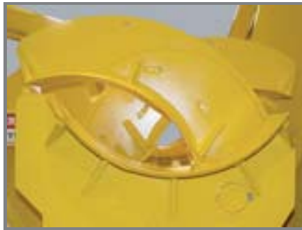
4 - Knives, Made Of Hi-Alloy Wear Hardening Steel, For Long Life.
