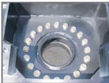
Strong Rotation Bearing Bolts, (3/4 L-9).
