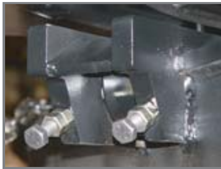
Strong Roller Adjustment, Designed For Easy Maintenance Access.
