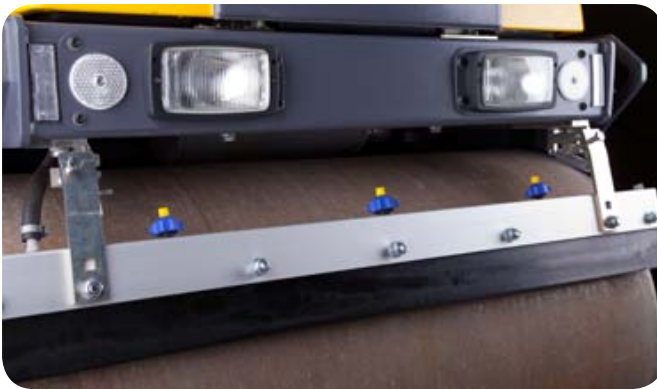
Pressurized sprinkler system with a powerful water pump and with self draining sprinkler tubes and nozzles.
