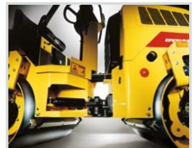
Maintenance-free articulated joint and steering cylinder.
