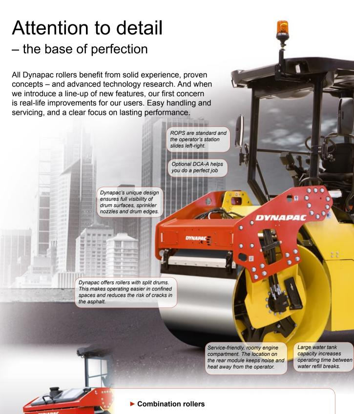
The CC224HF and CC234HF can be ordered in Combi versions to further improve top layer finish. The Combi module is placed rear and is combined with offset steering. Standard equipment includes an emulsion tank, sprinkler nozzles, handles and footsteps for tank filling, access and safety, quick-release of scrapers and cocoa mats for easy cleaning. Heat shield is available as option.
