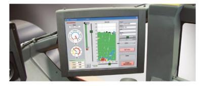
The Dynapac Compaction Analyzer for Asphalt (DCA-A) is the perfect tool for operators. It provides accurate time information about the rolling operation, allowing the next pass to be planned, taking into account the asphalt temperature of each pass.
