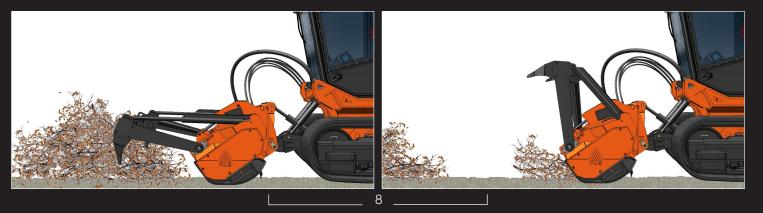
8. New raker teeth on guard frame. To drag logs and material and can be used as guide pins.
