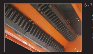
6. Easily interchangeable counter blades (up to 3 lines), made of wear-resistant steel
