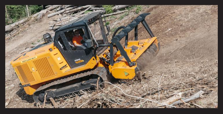
The FAE **200/U** mulching head for PT-300 is the ideal choice for any land clearing job, including vegetation management and ROW clearing. It is built very robust to be used for very heavy-duty jobs. Due to its spiral rotor design it reduces vibrations, absorbs less power, and increases productivity.
