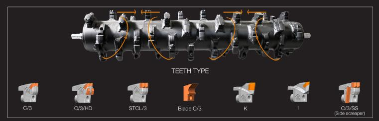
The double spiral rotor design ensures even distribution of the power over the entire width of the rotor, limits stresses to the structure, absorbs less power and enables even distribution of the mulched material. Wide range of interchangeable teeth are available for different working conditions.
