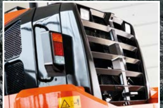
Optional wide fin radiators enhance durability.
