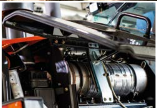
NO DPF SCR system reduces emissions.
