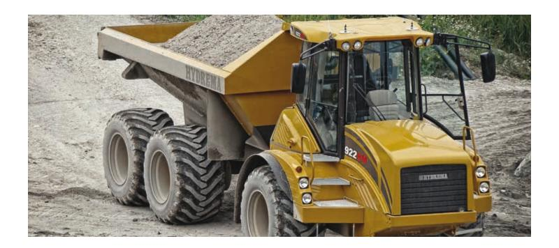
The variable engine fans provide cooling as needed, which makes it both very fuelefficient and quiet. The advanced transmission shifting system guarantees high stability with smooth gear shifts. This prevents wheel slipping and provides the best torque.
