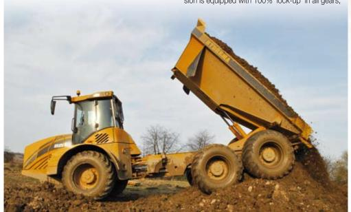
giving direct drive which bypasses the converter, and thus minimal energy loss. The specially optimized software ensures the best possible connection between the engine and the transmission in any condition.
