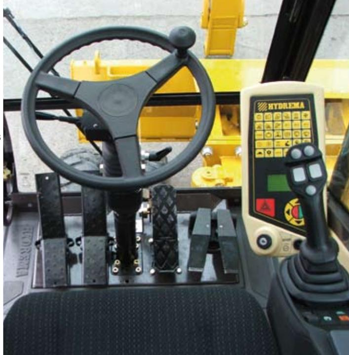
The joysticks are integrated into the soft-touch armrest which again are directly integrated into the seat - consequently the movements follows the operator. The layout of the computer-controlled
