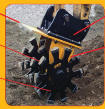
Featuring an unique, patent pending locking wheel removal design and specially designed, staggered pads, the IHW Series is ideally suited for cohesive and clay soil environments where vibratory plate methods may not achieve optimum results. Simple to install and operate, the IHW Series requires no special hydraulic con nections and is available in a wide variety of models and width sizes to accommodate most excavator brands.
