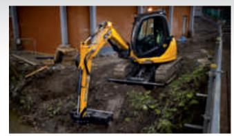
the robust build of a JCB compact excavator the new 8085 ZTS is a true work horse. Furthermore, versatility is ensured by the wide range of buckets and new electronic proportional auxiliary control option – enabling operators to use a wide range of hydraulic attachments to suit the increasing demands of the compact excavator market.
