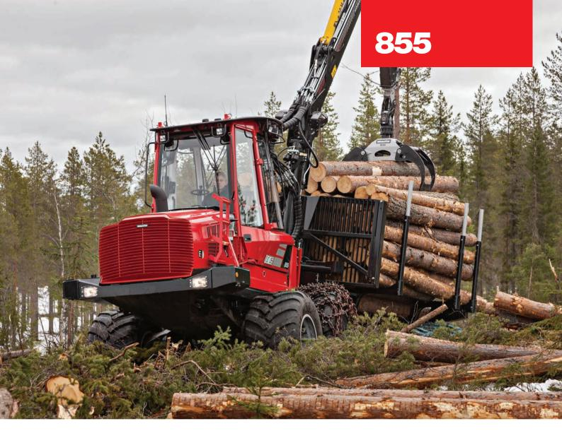
based engine, which both minimizes emissions and maximizes fuel efficiency. To that you can add improvements in terms of both an impressive torque and cleaner engine oil. Service costs are cut further by the addition of tight-seal ORFS couplings and a minimized number of lubrication points.
