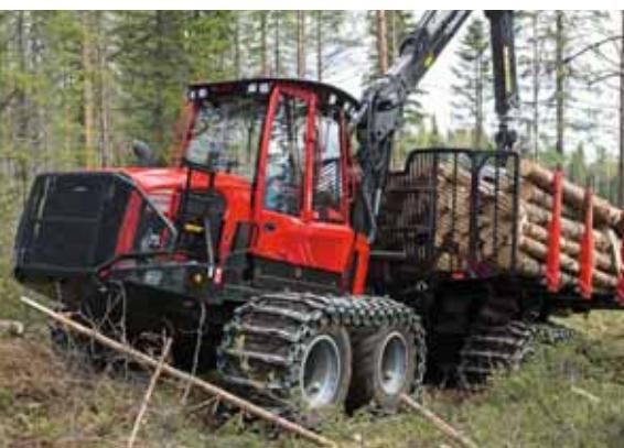
The ingenious HST transmission, with an underlying tractive force of 214 kN, produces improved performance thanks to a unique interaction with the control system and engine.
