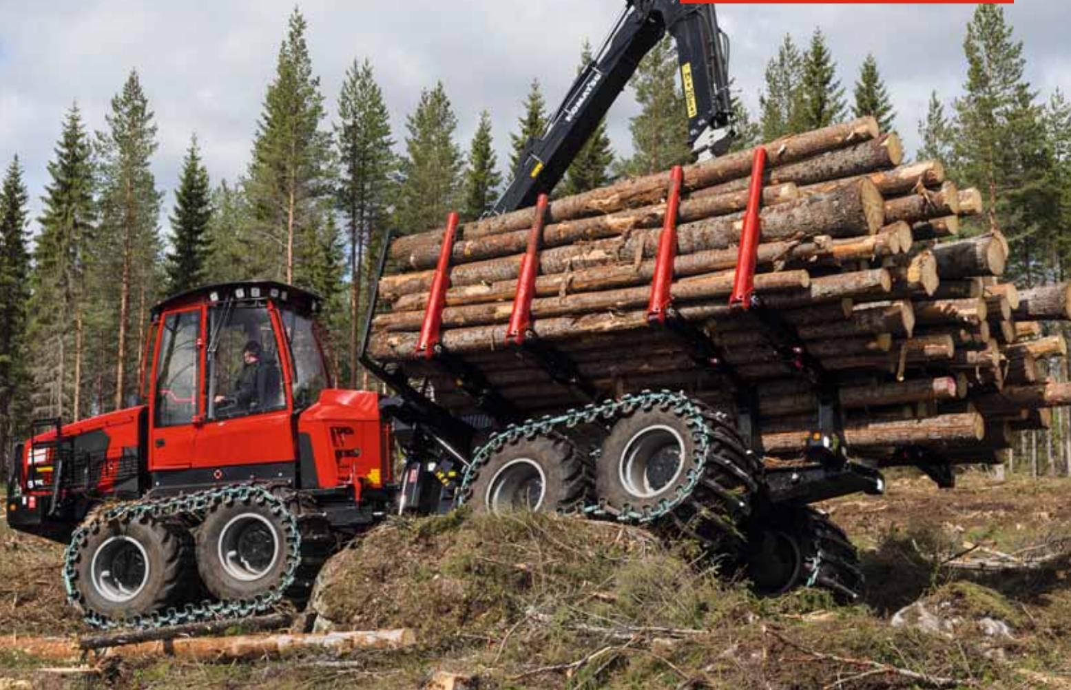
latest environmental requirements. The powertrain provides its highest torque at low engine speeds and automatically adapts to changes in engine load due to terrain, obstacles, inclines and crane loads. The ingenious transmission solution delivers optimum interaction between engine, transmission and control system, making the machine particularly manoeuvrable.
