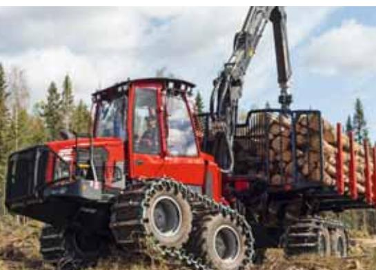
Thanks to its optimal balancing, the Komatsu Comfort Bogie – our portal bogie – provides superb ground clearance and off-road driving properties.
