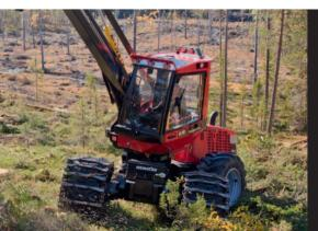
Leveling of both the cab and boom, and linkage with the swing axle for optimum reach and stability.
