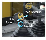
the blade will adjust pitch position from dig to dump with no additional lever movements. The blade pitch control can be set to automatically return to the digging position when in reverse.
