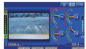
Hybrid system temperature gauge
