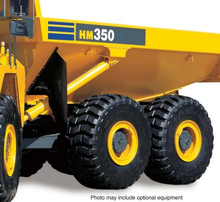
High capacity, reliable, continuously cooled, wet type multiple-disc brakes and retarder combination.
