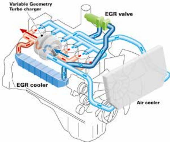
**Komatsu Variable Geometry Turbocharger (KVG) system**
