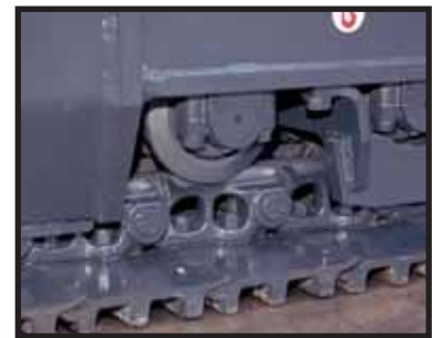
Track link with strut The PC160LC-7 uses track links with struts, providing superb durability
