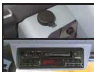
12-Volt power supply and (optional) radio cassette
