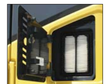
External air conditioner filter
