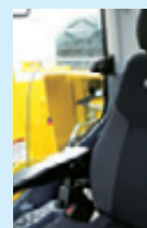
One-touch storable front window lower glass
