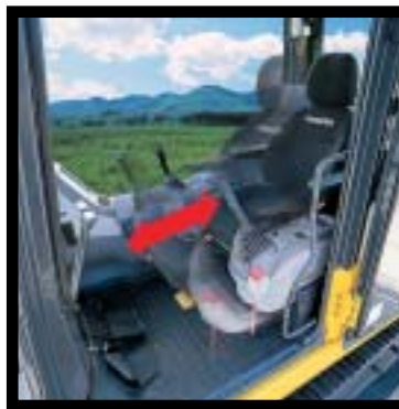
Seat Sliding Amount: 340 mm 13.4", increased 120 mm 4.7"
