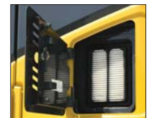
External air conditioner filter
