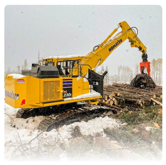
Forestry processing applications are a challenging task in often difficult environments, and Komatsu forestry excavators are built specifically to tackle these situations. Rugged front work equipment, high and wide undercarriage, powerful swing system and special cooling system promote high performance in demanding processing applications.
