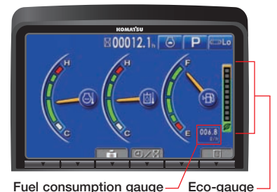
Fuel consumption gauge Eco-gauge
