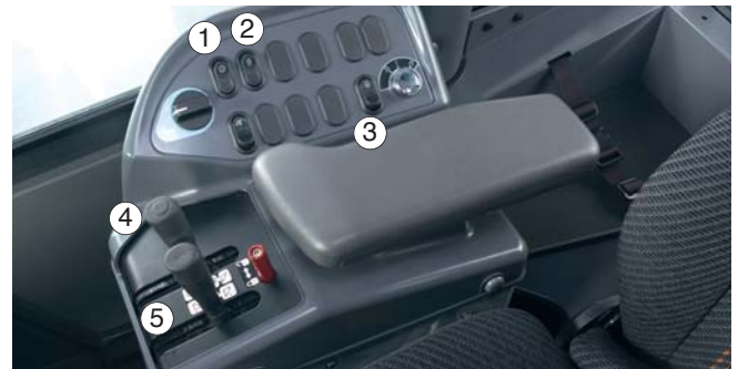
1: Cut-off ON/OFF switch 2: Cut-off adjustment switch 3: Fan reverse ON/OFF switch 4: Boom control 5: Bucket control
