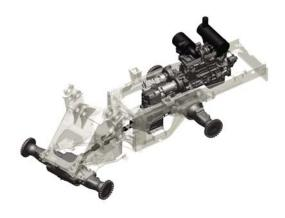
**Maintenance-free** fully hydraulic wet multi-disc service and spring applied, hydraulically released wet multi-disc parking brakes results in lower maintenance cost and higher reliability
