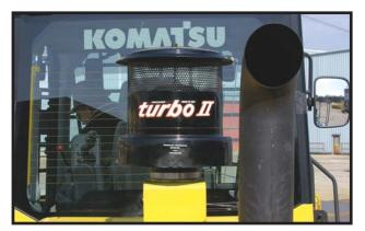
**Centrifical Air Pre-Cleaner** Donaldson and Turbo II brand pre-cleaners are available for increased purification of the engine inlet air.
