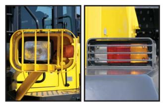
Heavy-Duty Head Light and Tail Light Guards Headlights are moved inward and metal guarding protects the headlights and tail lights from debris that may break or damage the lenses.
