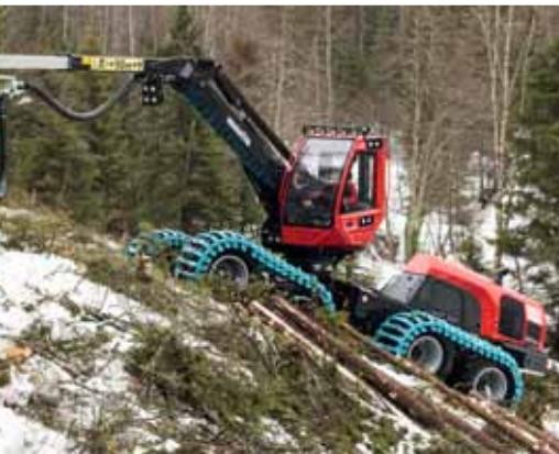
The cab levelling function means that you are always seated horizontally and that don't need to stretch and strain to maintain a good seating and working position.
