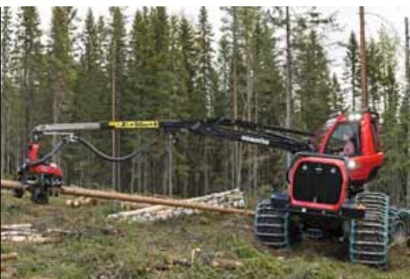
The cab and the crane can be rotated 360°. Large work area increases the timber concentration and productivity for the forwarder.
