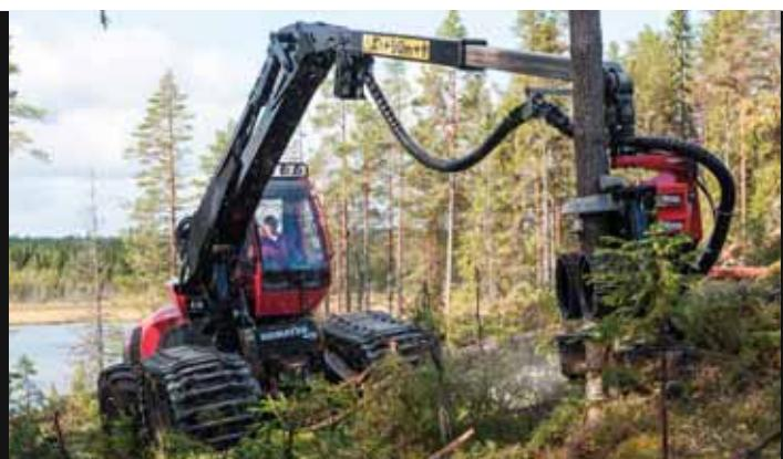
The unique solution with the crane placed in the middle of the machine and the coupling between the tilt cylinders and the swing axle provide superior stability.
