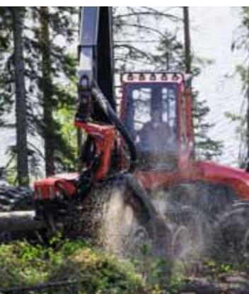
Always perfect visibility. Thanks to the crane's placement to the side of the cab, you always have optimal visibility of the head whether it's close to or far from the cab.
