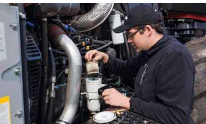
New service advantages – everything from improved access to filters and separate hatches for refilling diesel and hydraulic oil to a cassette system for faster valve adjustment.
