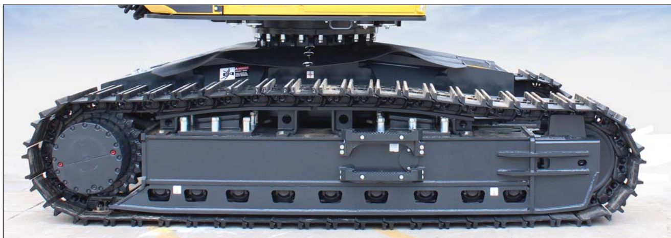
Rugged Komatsu Undercarriage with 9 Large Capacity Rollers; Choice of Track Sliders or Carrier Rollers
