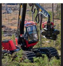
High traction, which together with the unique bogie, provides optimum performance and maneuverability in steep terrain or on soft/wet ground.
