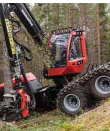
The cab levelling function means that you are always seated levelly and don't need to stretch and strain to maintain good posture.
