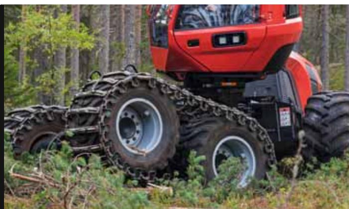
Komatsu Comfort Bogie – our unique portal bogie – provides superb stability, ground clearance and manoeuvrability.
