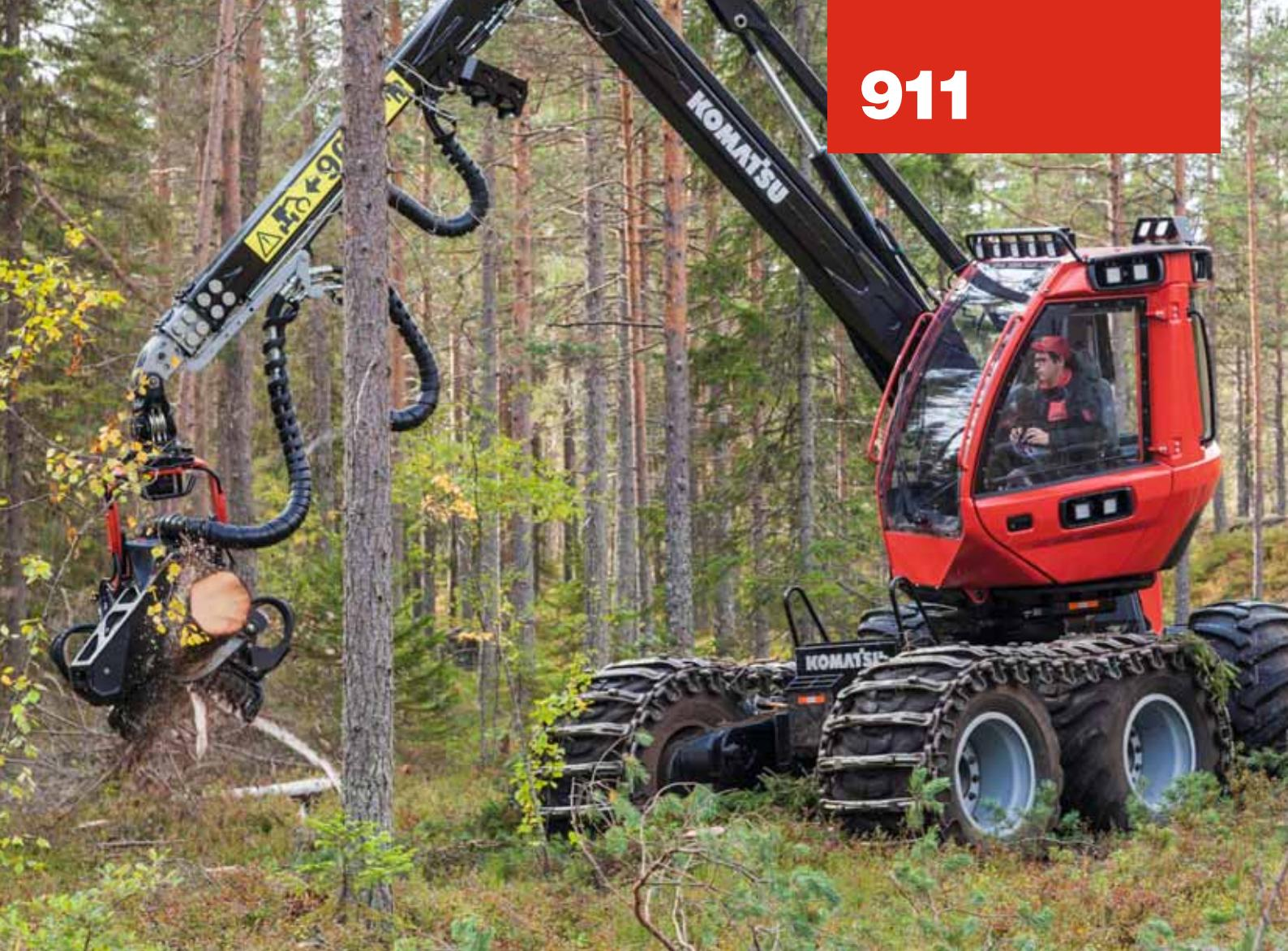
diesel-guzzling engine power. Instead, you save time by, for example, being able to slew and feed simultaneously with maintained pressure and flow. What's more, with a full 360 degrees of cab rotation you can process more from the same spot, which optimises forwarding. As expected, you can enjoy Komatsu's superior stability thanks to the unique crane placement and coupling between the tilt cylinders and swing axle.
