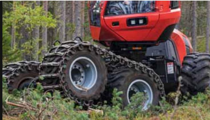
Komatsu Comfort Bogie – our unique portal bogie – provides superb stability, ground clearance and manoeuvrability.
