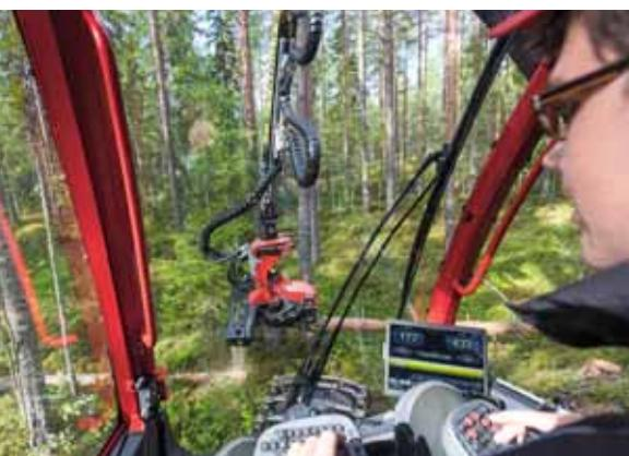
New large and noise-reducing cab with larger windows that provide superior visibility upwards, downwards and to the rear.
