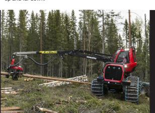
The cab and the crane can be rotated 360°. Large work area increases the timber concentration and productivity for the forwarder.
