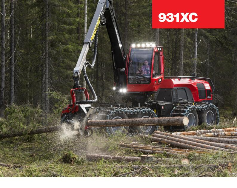
combined the suspended rear axle with a bogie mounted on the single axle. This produces unique driving characteristics, and the manner in which the machine follows any unevenness in the terrain is unparalleled. A crane with higher slewing force and the machine's high ground clearance are other properties that are useful in steep, tough terrain.
