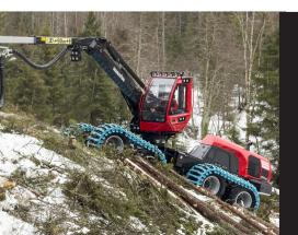
The cab levelling function means that you are always seated horizontally and that don't need to stretch and strain to maintain a good seating and working position.
