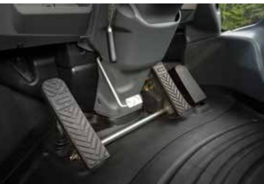
(l-r) Inching/Brake Pedals, Accelerator Pedal
