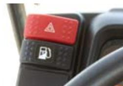
The operator can select either "Power" or "Fuel Efficient" engine mode. Power mode provides added power for extreme applications. Fuel Efficient mode offers better fuel economy for standard applications.
