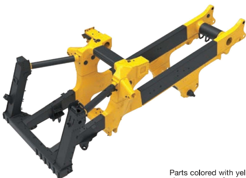
Parts colored with yellow show cast-steel components.
