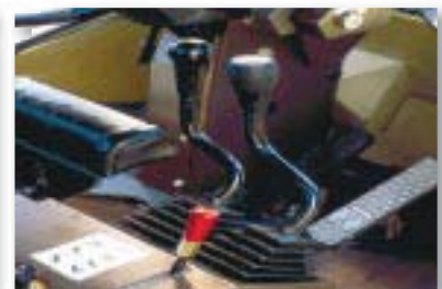
Boom and bucket controls with kick-down switch
