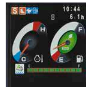
DEF tank level gauge
