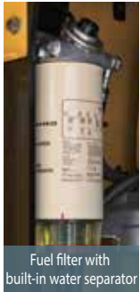
Fuel filter with built-in water separator
