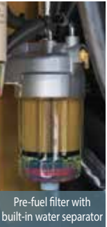
Pre-fuel filter with built-in water separator
