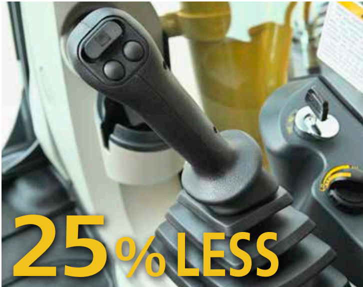
It takes 25 % less effort to work the operation lever, which reduces fatigue over long working hours or continuous operations. *Compared to SK350LC-9 model
