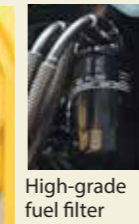
Pre fuel filter with built-in water separator
