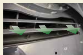
Offset duct slow down exhaust
