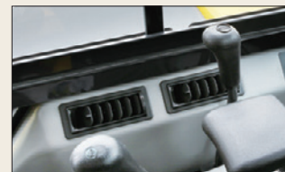
Heater with fresh air vents
