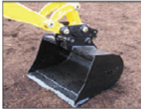
Ditching Grading Bucket
