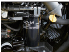
Large secondary fuel filter
