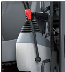
Lever shown in lock position
