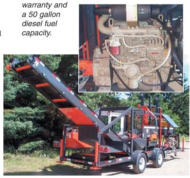
The Model 2020CSC is a highly mobile machine with tandem axles, single tires, electric brakes and a pintle hitch for towing.
