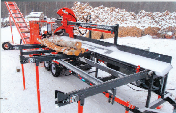
Rugged Duty tubular frame, Heavy Duty Log Deck with Roller Chain
