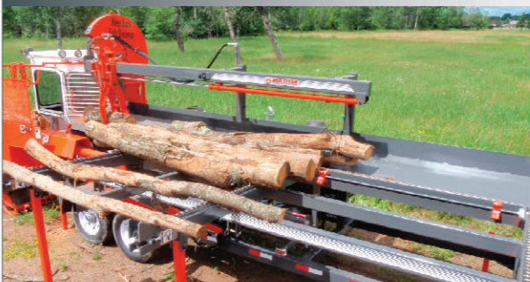
Rugged Duty tubular frame, Heavy Duty Log Deck with Roller Chain
