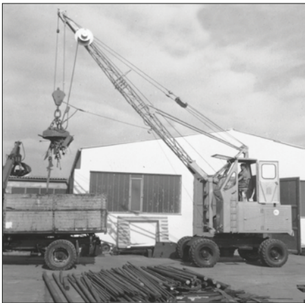
1962: Rope-driven S833 with elevated operator cab
